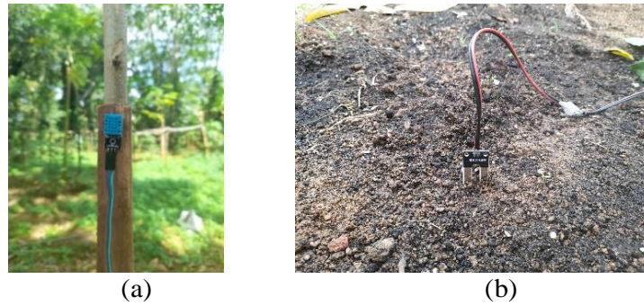
Figure 8 (a): On field attachment of Arduino DHT 11 sensor, 8 (b) soil moisture level sensor.
