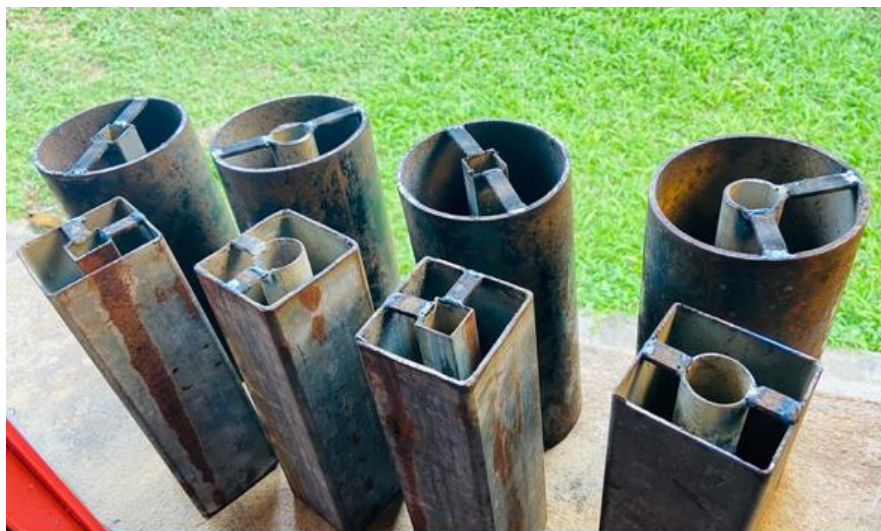
Figure 4 CFDST steel specimens in circular and rectangular sections are ready to undergo testing procedures.
