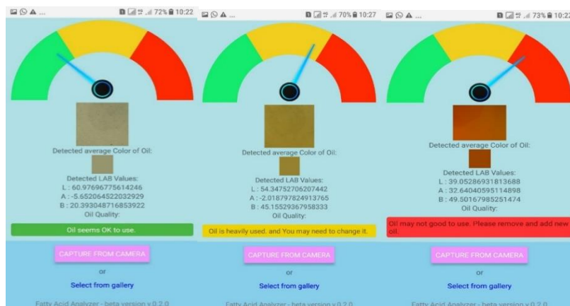
Figure 4: Screenshots of the Results Interface Showing Three Stages (Fresh, Intermediate, Rejected) of Frying Oil in the Mobile Application.
