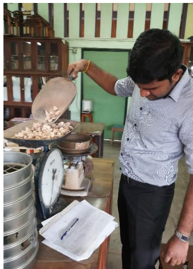
Figure 3: Preparation of limestone aggregate sample.
