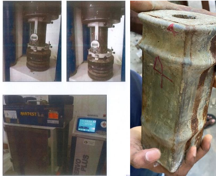
Figure 5 Axial compression of specimen and deformed shape.
