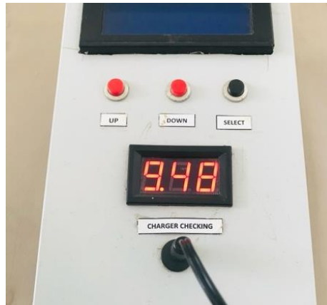
Figure 6: Voltage Measurement of a DC Charger
