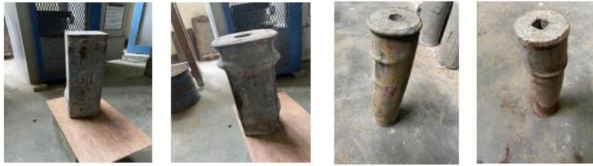
Figure 7 Deformed shape of the tested specimens.
