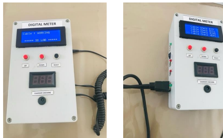
Figure 9: RJ9 & HDMI Cable continuity checking
