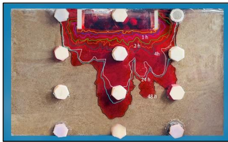
Figure 6: Contaminant flow path of C50:F50
