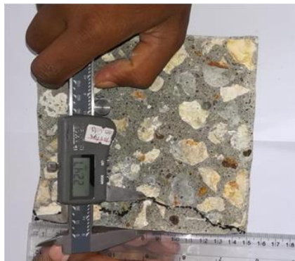
Figure 8: Measuring depth of water penetration in Fly ash-based limestone aggregate concrete cube sample.
