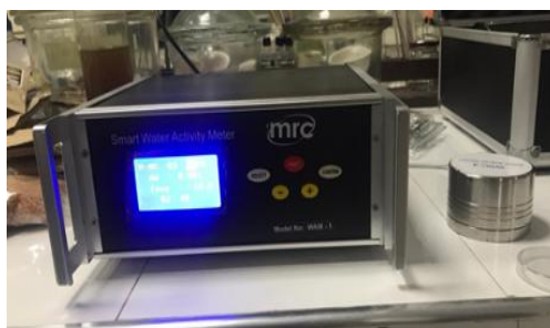
Figure 2. Water activity meter (mrc WAM-1) at Food research unit, Department of Agriculture, Peradeniya
