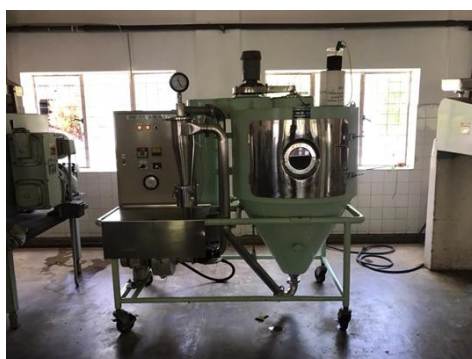
Figure 1. Spray dryer (Ohkawara kakohki L-8) at Food research unit, Department of Agriculture, Peradeniya
