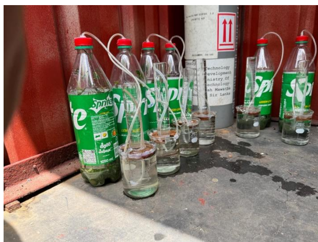
Figure 1: Experimental Digester setup
