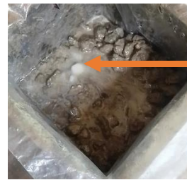
Figure 3: Photograph of capsules incorporated during sample preparation
