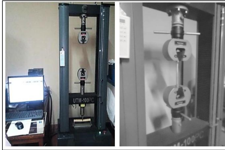
Figure 4: UTM Machine (UTM-100PC-Australia) and Loading setup
